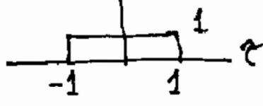
NO  $\left\{ \begin{array}{l} 1. x(\tau) = x(-\tau) \checkmark \\ 2. x(0) \geq x(\tau) \checkmark \\ 3. \mathcal{F}\{x(\tau)\} \text{ is a positive and negative going function.} \end{array} \right.$
